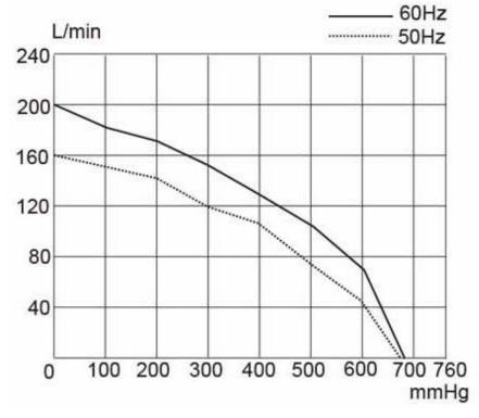
$\frac{\textbf{FLOW CONVERSION}}{\text{L/M X } 0.035} = \text{CFM}$
