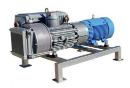
US VACUUM TorrVac vacuum pumps are Single stage Aircooled Rotary Vane Direct drive vacuum pumps capable of producing an ultimate vacuum of 29.9" Hg (0.5 mm Hg) . The pumps are rugged and designed for continuous operation in industrial applications.
